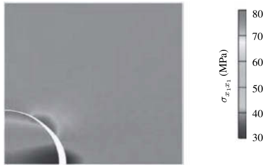
Figure 15.26 Contour plot showing \sigma_{xx} in the fibre–epoxy system at \bar{u} = 0.165 \mu\text{m} using the 128 elements discretisation. The displacements are amplified by a factor of 10 (Verhoosel et al. 2011a)
