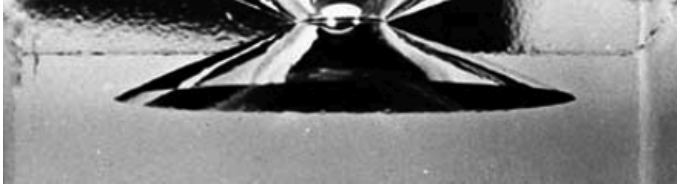
Figure 4.11. The Hertzian cone crack under spherical indenter, as experimentally observed (taken from [ROE 56])
