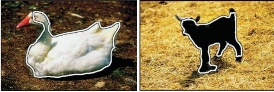
Figure 15.5 Segmentations of example images using invariant features. Note that the backgrounds with cast shadows are well segmented, that is, disregarding the cast shadows. Source: Reprinted with permission, © 2005 Elsevier.
