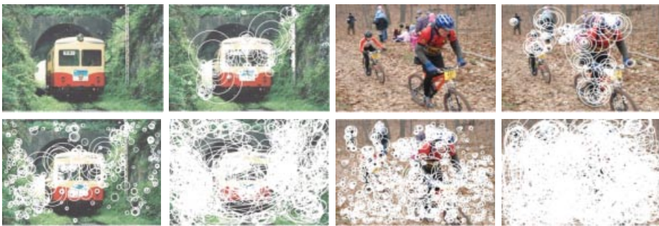
Figure 1.2 Visual exploration is based on the paradigm to divide the images into meaningful parts from which features are computed. Saliency point detection is applied first from which color descriptors are computed. Then, machine learning is applied to provide classifiers for object recognition.
