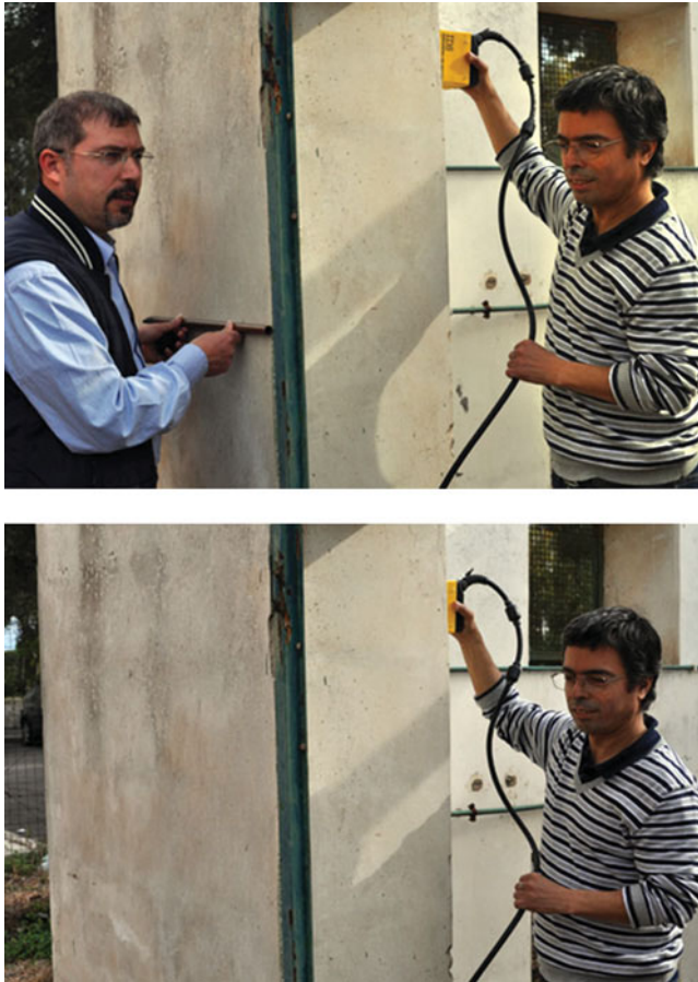
Figure 2.1. Upper panel: A metallic road is placed horizontally on the other side of the prospected wall. Lower panel: The metallic road is removed. The antennas have been moved in both cases downward along a vertical line.
