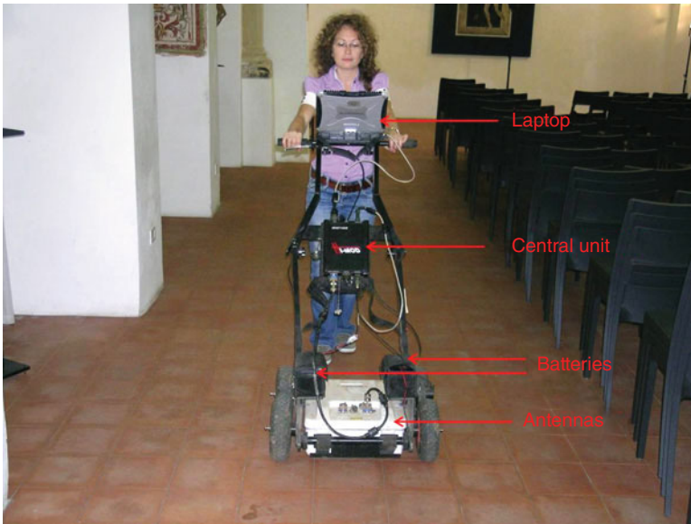
Figure 1.2. Photograph of a GPR (a Ris Hi Mode system) equipped with a double antenna at 200 and 600 MHz antenna.
